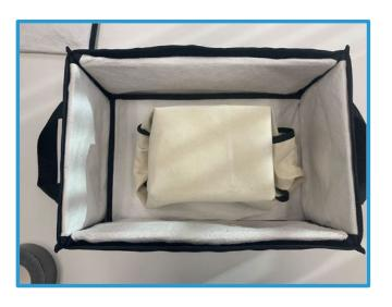
Wrap the fire-resistant blanket over the battery pack and tuck in all exposed corners or gaps.
