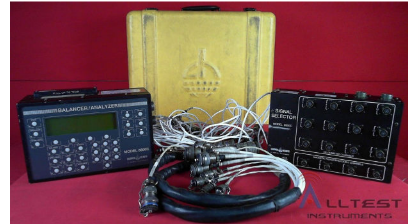
Typical carry-on equipment that plugs into aircraft to download vibration data during flight operations in the track and balance procedure
