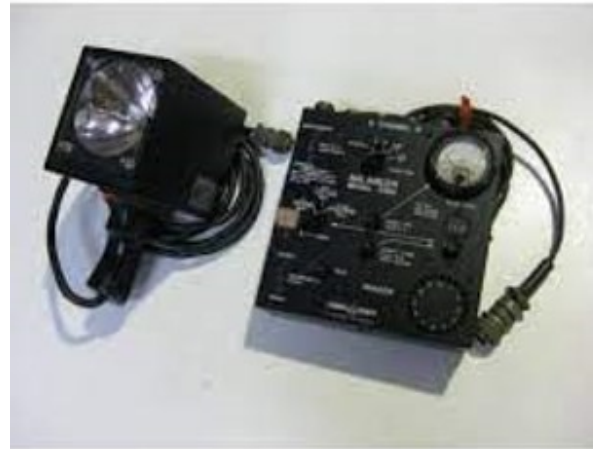
Strobe light used to “find” a moving blade target to illuminate the heavy side of the imbalance. Developed in the 1960’s but still in play today
